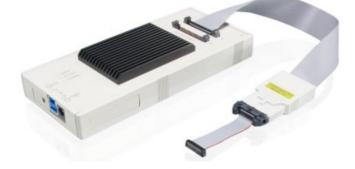
The unused connector (in the image) is used for an optional Analogue Probe which can be used to measure voltage and current and profile the energy use of application code. When used in conjunction with the ETM trace, the amount of power each function uses can be measured and algorithms can be adjusted to be less power hungry, if required.
