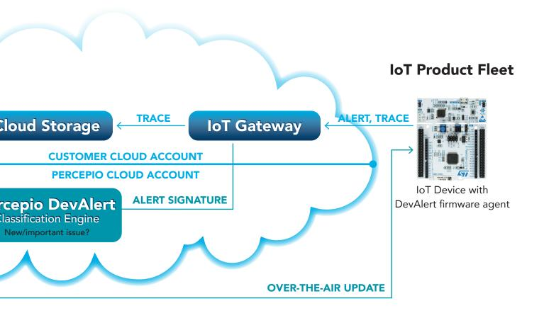
on 15 years of experience in RTOS tracing and is 4-8x more memory efficient than traditional RTOS tracers – only 4 KB is needed to store a trace with up to 1000 software events. The efficient trace encoding is important for three reasons – it allows us to collect traces of sufficient length from memory-constrained IoT systems, it reduces the upload time to a fraction of a second and it minimizes the cloud-side operational costs of DevAlert messaging and storage.
