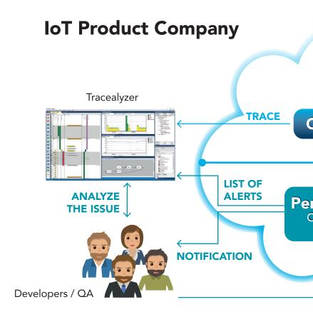
Devices with secure IoT connectivity enable us to think about firmware development in a new way. The traditional code – test – debug cycle remains as important as it's always been, but since we know from research and experience that some bugs almost certainly remain in deployed code, why not use the connectivity for automatic error reporting from deployed devices?
